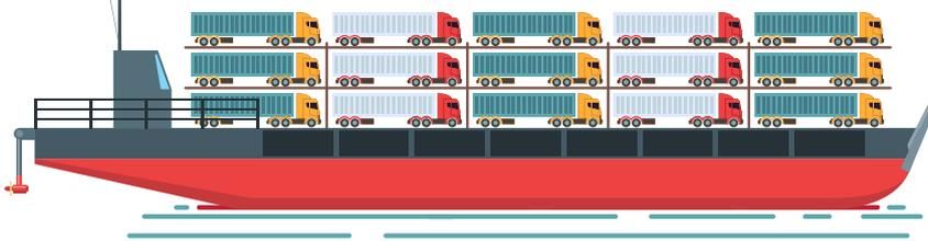
A convoy, made of two industrial barges of 80 meters by 11,4 meters each and a pusher (total length of 185 meters) will be able to circulate by inland from Le Havre to Constanta, a Black Sea Harbor, and carry till 4.400 tons of goods each, replacing in this way 220 trucks. A convoy departing every 30 minutes will be equivalent to the circulation of one truck every 8 seconds.
