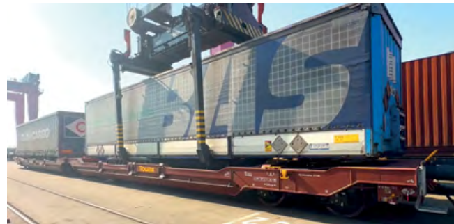
Touax Pocket wagons for transport of semi-trailers
